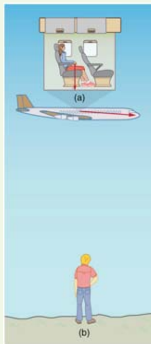
Figure 3.49 The motion of a coin dropped inside an airplane as viewed by two different observers. (a) An observer in the plane sees the coin fall straight down. (b) An observer on the ground sees the coin move almost horizontally.
