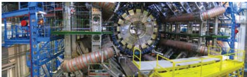
Figure 4.27 The world's largest particle accelerator spans the border between Switzerland and France. Two beams, traveling in opposite directions close to the speed of light, collide in a tube similar to the central tube shown here. External magnets determine the beam's path. Special detectors will analyze particles created in these collisions. Questions as broad as what is the origin of mass and what was matter like the first few seconds of our universe will be explored. This accelerator began preliminary operation in 2008. (credit: Frank Hommes)
