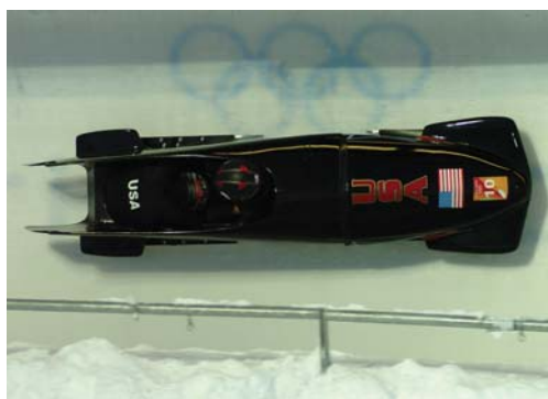
Figure 5.7 From racing cars to bobsled racers, aerodynamic shaping is crucial to achieving top speeds. Bobsleds are designed for speed. They are shaped like a bullet with tapered fins. (credit: U.S. Army, via Wikimedia Commons)
