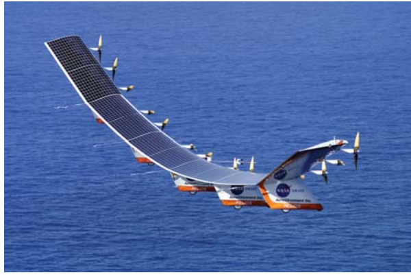
Figure 7.20 Solar energy is converted into electrical energy by solar cells, which is used to run a motor in this solar-power aircraft. (credit: NASA)
