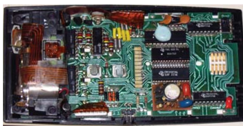
Figure 19.23 Energy stored in the large capacitor is used to preserve the memory of an electronic calculator when its batteries are charged. (credit: Kucharek, Wikimedia Commons)
