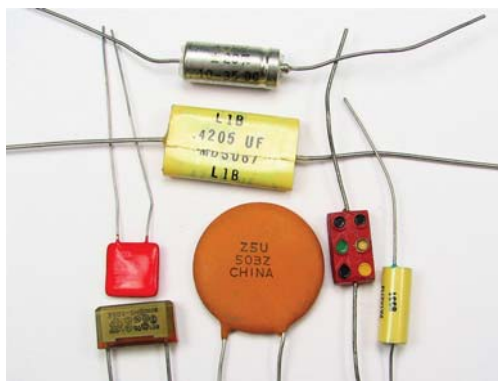
Figure 19.15 Some typical capacitors. Size and value of capacitance are not necessarily related. (credit: Windell Oskay)
