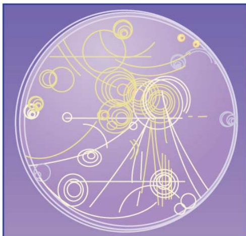
Figure 22.19 Trails of bubbles are produced by high-energy charged particles moving through the superheated liquid hydrogen in this artist's rendition of a bubble chamber. There is a strong magnetic field perpendicular to the page that causes the curved paths of the particles. The radius of the path can be used to find the mass, charge, and energy of the particle.
