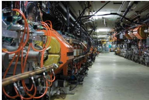
Figure 22.25 The Fermilab facility in Illinois has a large particle accelerator (the most powerful in the world until 2008) that employs magnetic fields (magnets seen here in orange) to contain and direct its beam. This and other accelerators have been in use for several decades and have allowed us to discover some of the laws underlying all matter. (credit: ammcgrim, Flickr)
