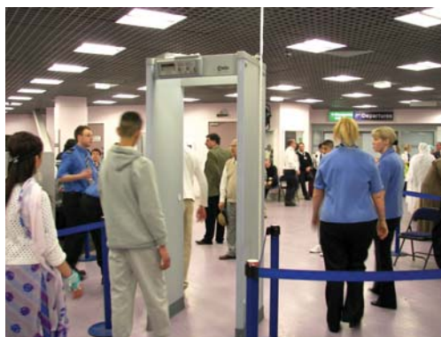
Figure 23.43 The familiar security gate at an airport can not only detect metals but also indicate their approximate height above the floor. (credit: Alexbairds, Wikimedia Commons)
